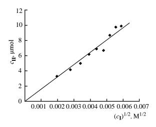
Quantity of carbonyl protein fragments determined as 2,4-dinitrophenylhydrazones ( $c_{\rm II}$ ,  $\mu{\rm M}$ ) vs. square root of albumin concentration ( $c_{\rm I}$ ,  ${\rm M}^{1/2}$ ). Aqueous phosphate buffer, pH 7.4,  $c_{\rm H_2O_2}$  4.21 × 10<sup>-2</sup> M,  $c_{\rm Fe^{2+}}$  1.84 × 10<sup>-4</sup> M,  $c_{\rm albumin}$  3.85–34.62  $\mu{\rm M}$ .
